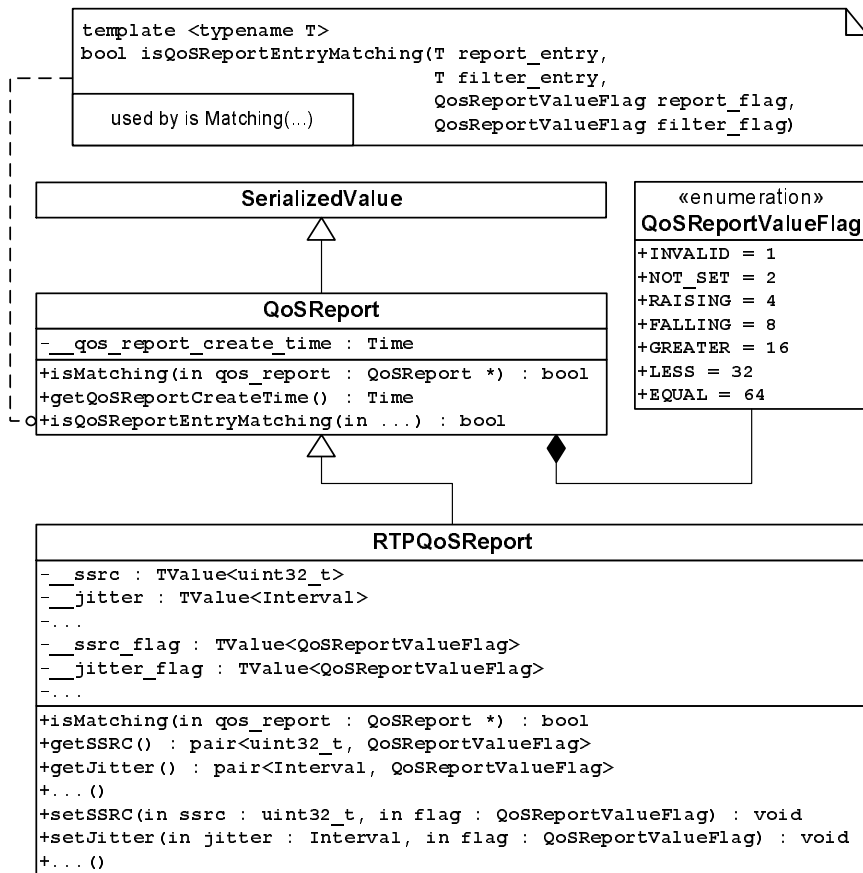
Figure 7.11: Class diagram of the class QoSReport.
